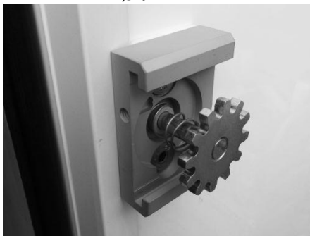
7 – With the Pinion and loose Spring in place, tighten Screws permanently
